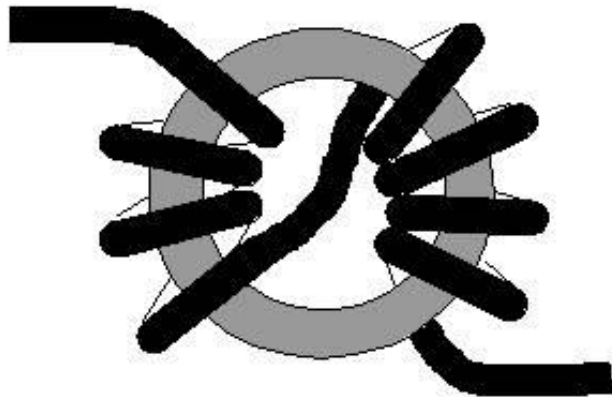
Common-Mode Choke of 4+4 Turns RG58 on 2*70mm Ferrite Core (RK1)
