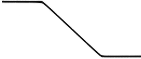
Fig. 5.22. Behaviour of the precision limiter circuit
