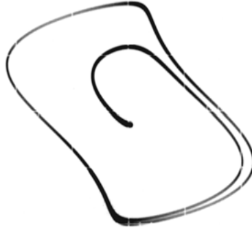
Fig. 6.17. Typical phase space plot of the solution of VAN DER POL's differential equation
