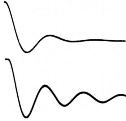
Fig. 8. Typical solutions for spring mass dampening. Top graph v = 0.6 \mu = 0.8 Bottom graph v = 0.8 \mu = 0.6 [5]
