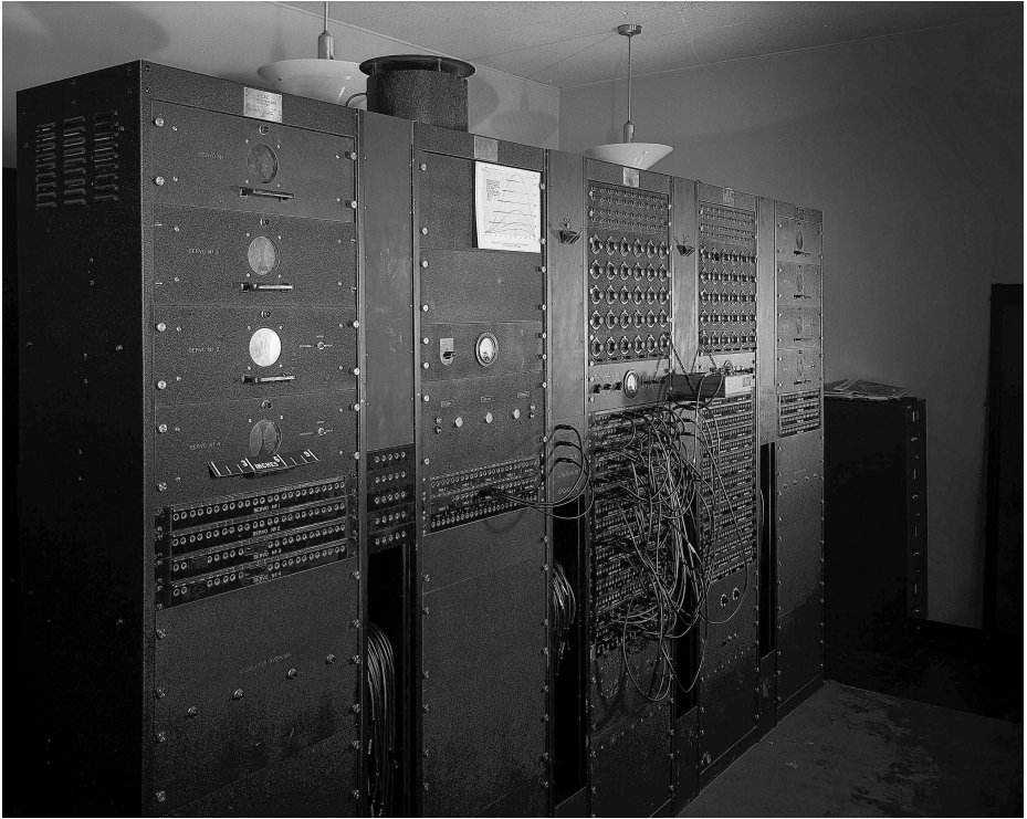
Fig. 13.51. Very early REAC analog computer (most probably a REAC 100) used by NACA as early as 1949
