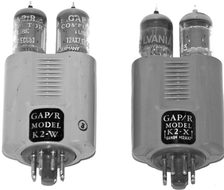
Fig. 4.8. K2-W and K2-X operational amplifiers (GAP/R)
