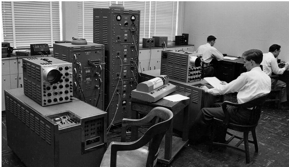
Fig. 10.13. Two MADDIDA systems in use at the Navy Electronics Laboratory (NEL, file number E1278)
