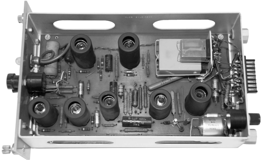
Fig. 4.12. Chopper-stabilised operational amplifier (Solartron)
