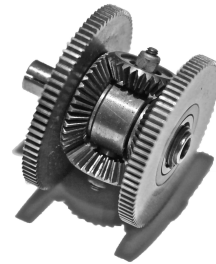
Fig. 2.10. A differential gear from the dead reckoning computer PHI-4A-2 used in Starfighter jets
