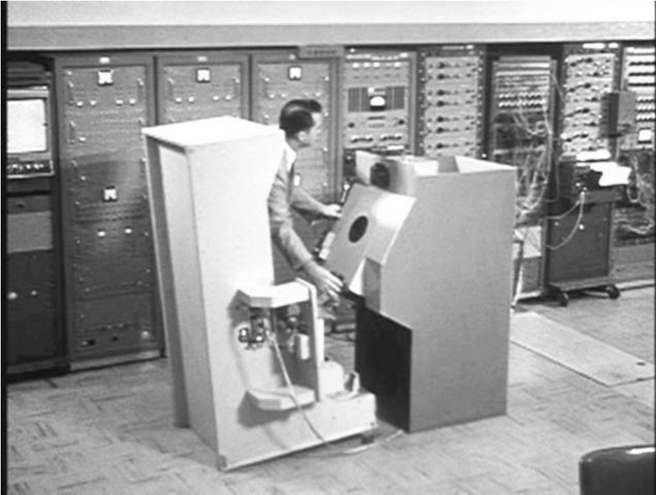
Fig. 13.68. Analog computer setup used during the development of the Mercury control stick (author's archive)
