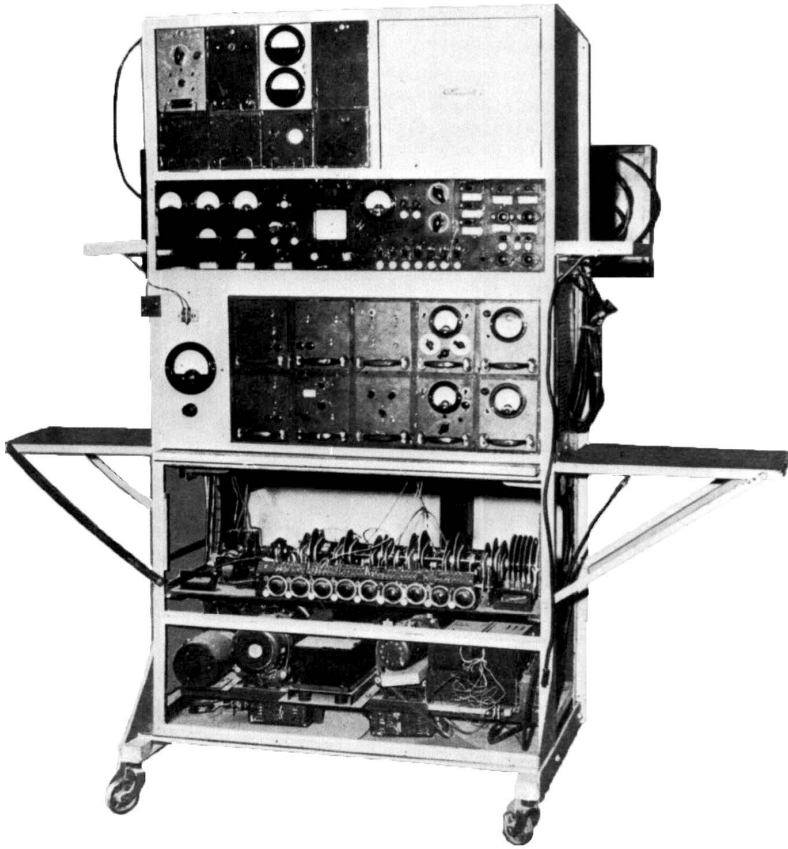
Fig. 3.16. HOELZER's analog computer for rocket motion simulation as it was found after World War II (source: NASA, Marshall Space Flight Center)
