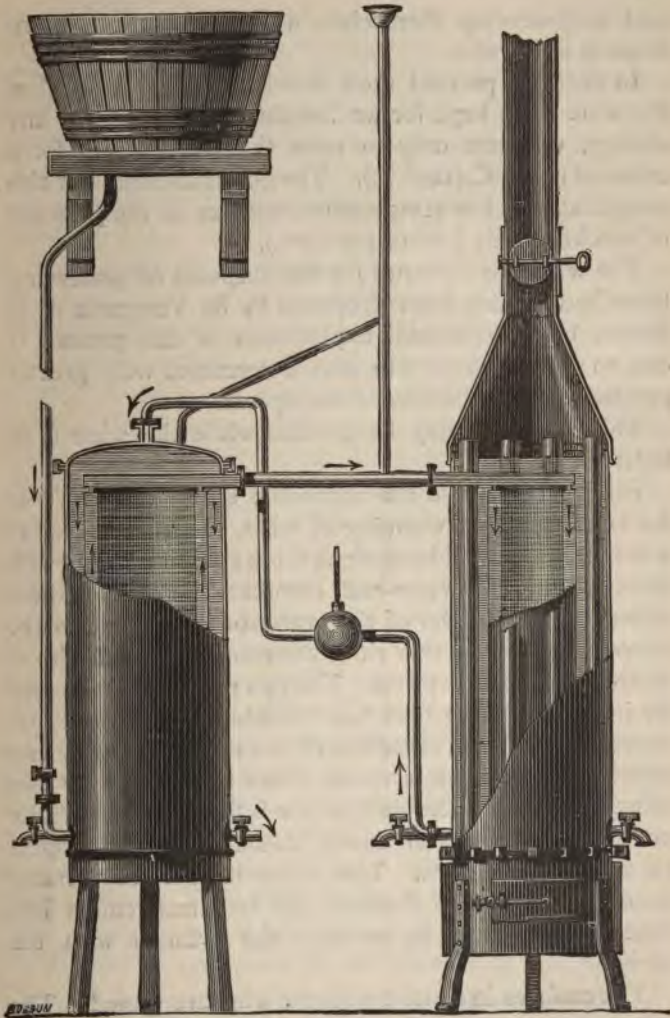
FIG. 23.—Giret and Vinas' apparatus for warming wines.
