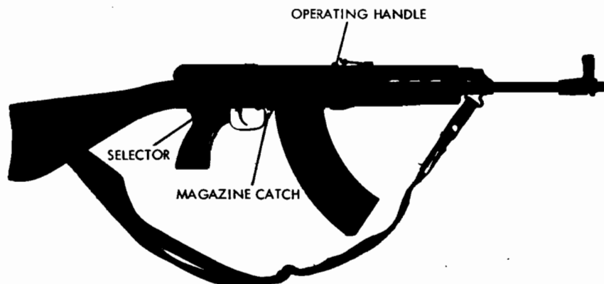
Figure 39. 7.62-mm Vzor 58P (Vz 58P) assault rifle.
