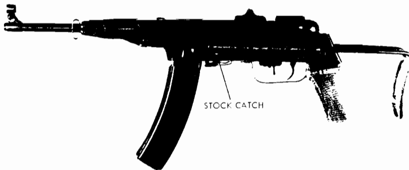
Figure 21. North Vietnamese 7.62-mm K-50 Modified submachinegun.
