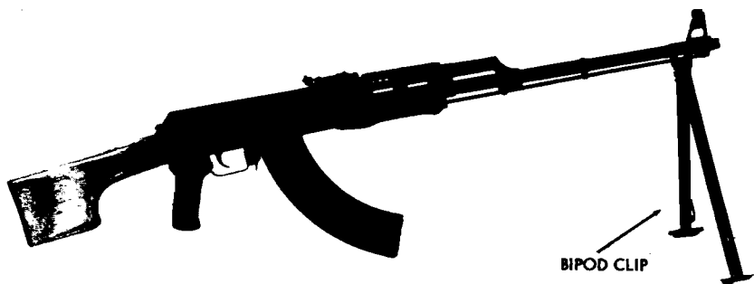
Figure 53. Soviet 7.62-mm Kalashnikov squad light machinegun (RPK).
