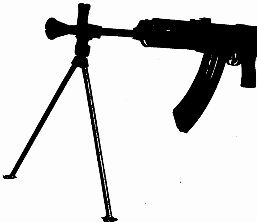
Figure 42. Vzor 58P assault rifle with flash hider and bipod.
