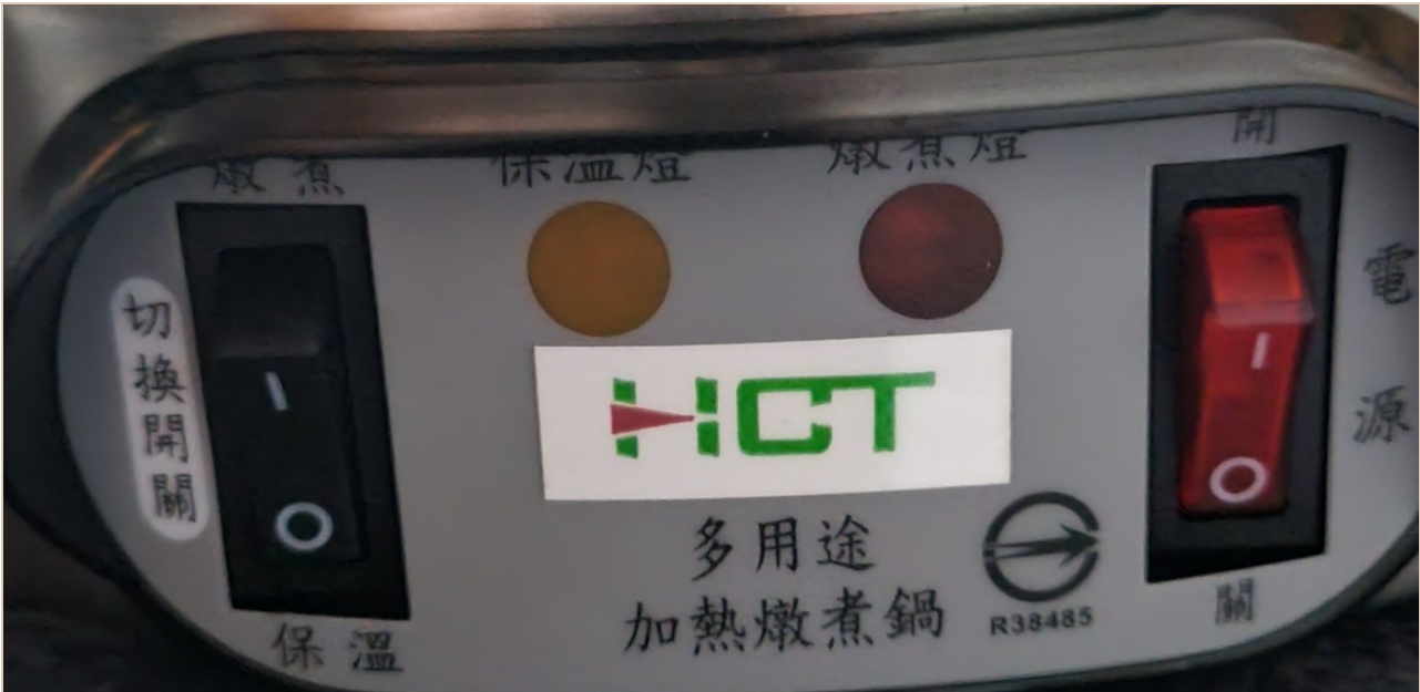
The panel as labelled on the machine. The badge reads 多用途加熱燉煮鍋 — “multi-purpose heating & stewing pot”. R38485 is the Taiwan BSMI commodity-inspection number.
