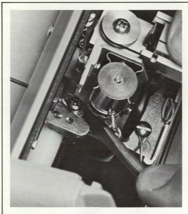
FIGURE 3-17. Y-AXIS GEAR TRAIN BACKLASH ADJUSTMENT
