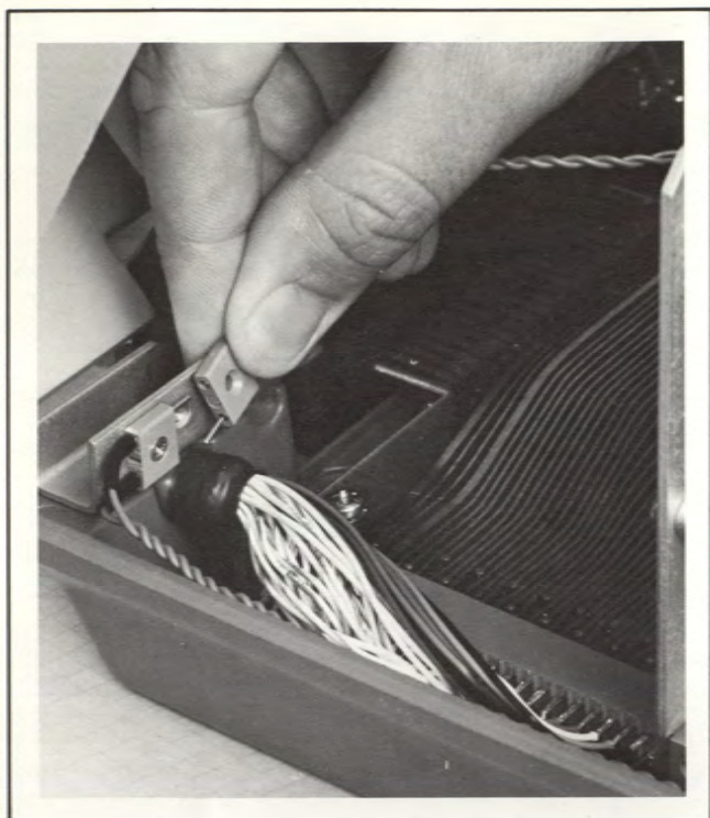
FIGURE 3-5. AUTOGRIP LEAD REMOVAL
