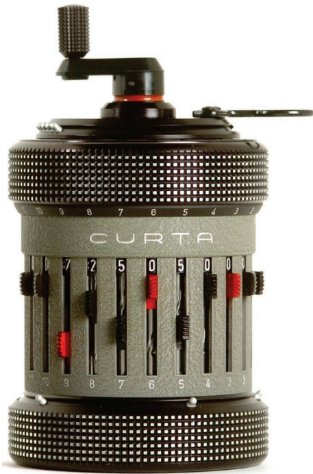
Figure 4. The Curta (Model 2). The Curta pocket calculator is a full-fledged four-function calculating machine (Credit: Liechtensteinisches Landesmuseum, Vaduz, picture: Sven Beham).
