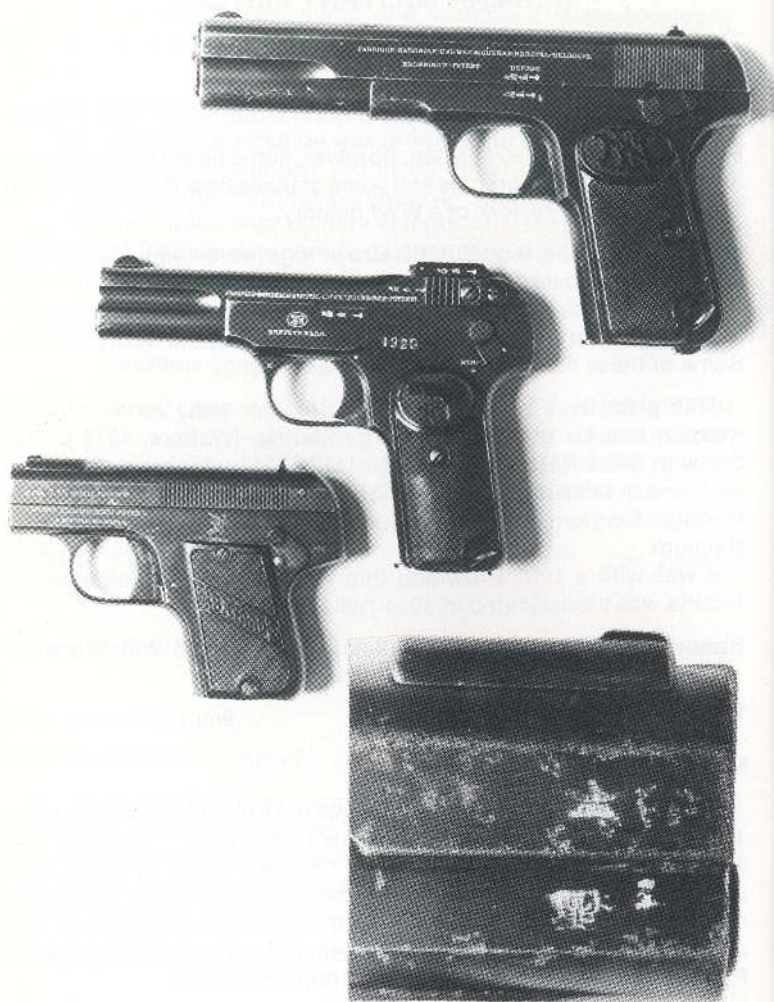
Figure 12. Pistols captured or manufactured in Belgium by or for the Imperial German military: top to bottom, 1903 Browning, 1900 Browning with German (Feuer and Sicher) safety markings and 1908 Bayard with Imperial German military stamps located on the right side of the frame and slide (see inset).
