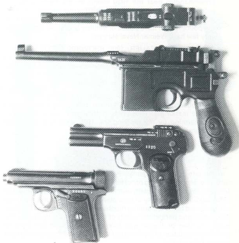
Figure 18. World War I military pistols with the 1920 "Weimar" stamp indicating reissue to the 100,000 man post war Reichswehr; top to bottom, P 08 1914/1920, M1896/16 Mauser which retains full length barrel and tangent sight, 1900 Browning with German (Feuer and Sicher) safety markings, 1913 Sauer. The P 08 is from the collection of E. Hildebrand and the Red 9 is from the collection of K. Weir.
