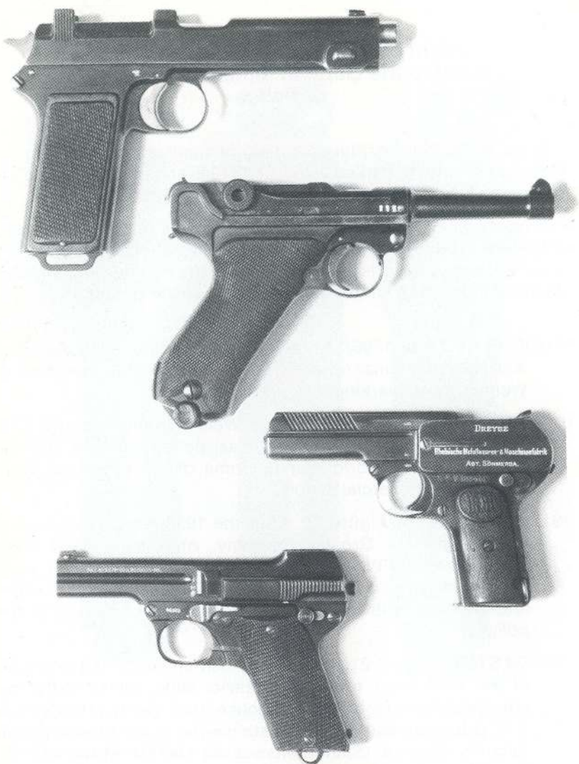
Figure 21a. Pistols with indications of postwar military or police reissue: top to bottom, Steyr Hahn with Nazi police acceptance Stamp-Eagle/L; P 08, 1914 dated, Erfurt with Steyr (1943) replacement barrel-Eagle/623; 1907 Dreyse with R.F.V. Nr. 3461 indicating Reichs Finanz Verwaltung issue; 1908/34 Steyr reworked for the Austrian police, in 1934, which became part of the Nazi police after the 1938 Anschluss.
