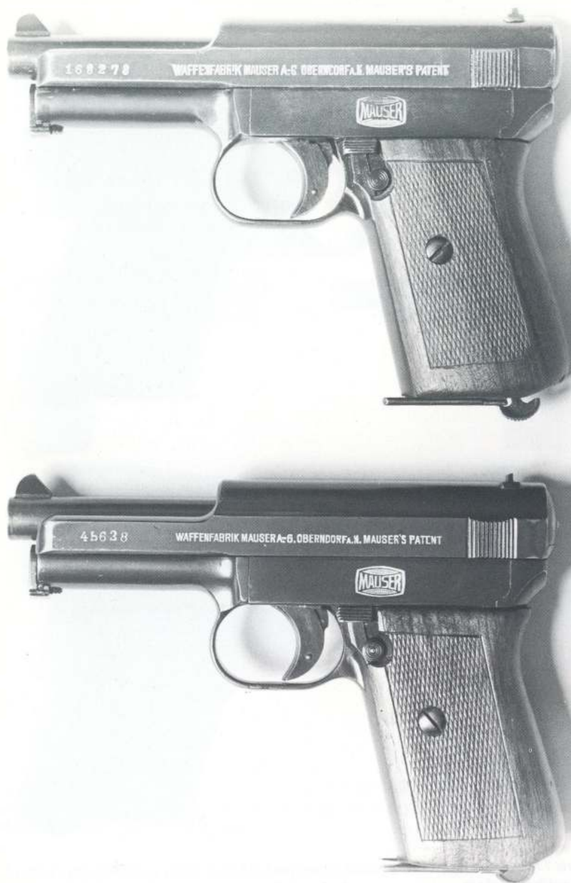
Figure 11c. 1914 Mauser Imperial variations: top, Imperial Army issue with military stamp near rear sight and "Prussian eagle" on trigger guard; bottom, wartime commercial model with military stamp near rear sight.
