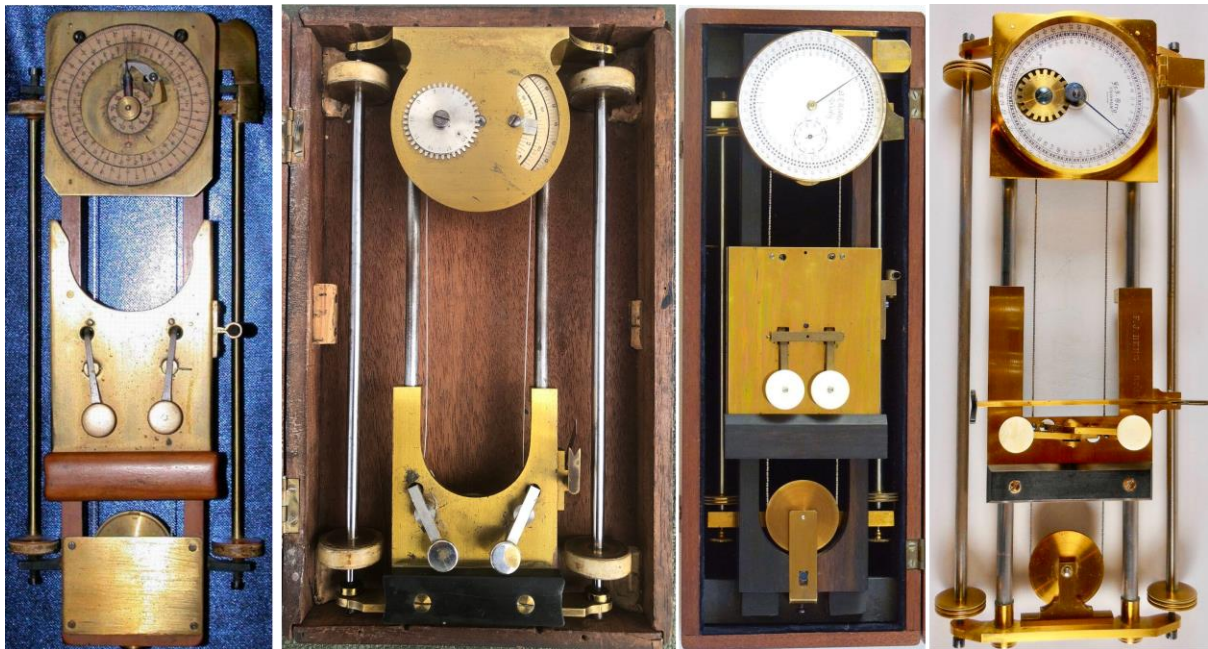
Figure 34: Mechanised harp planimeters from additional four different Swedish manufacturers. From left to right: Sköldin (according to the design by Liedbeck [And1876]), Ljungström, Köhler and Berg.
