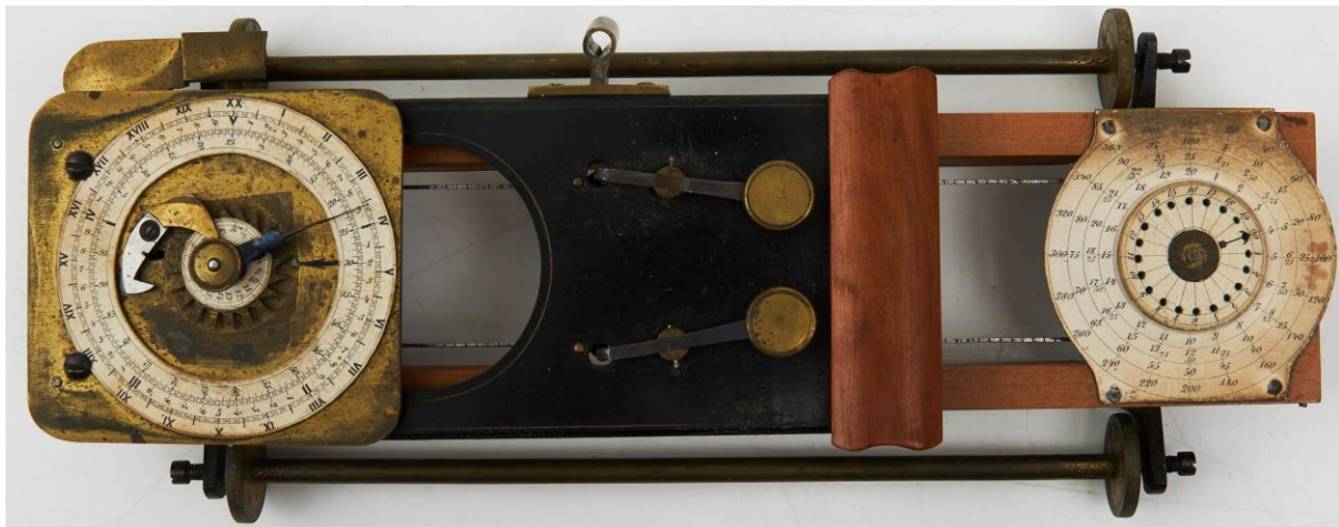
Figure 32: Liedbeck's mechanized harp planimeter, 1868, serial number 129. (Photo: Stockholms Auktionsverk)
